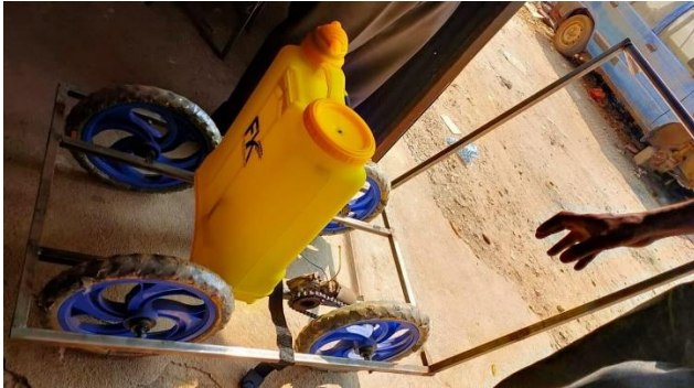
Fig 3: Electrically run Agriculture Sprayer Vehicle fabricate by our group
